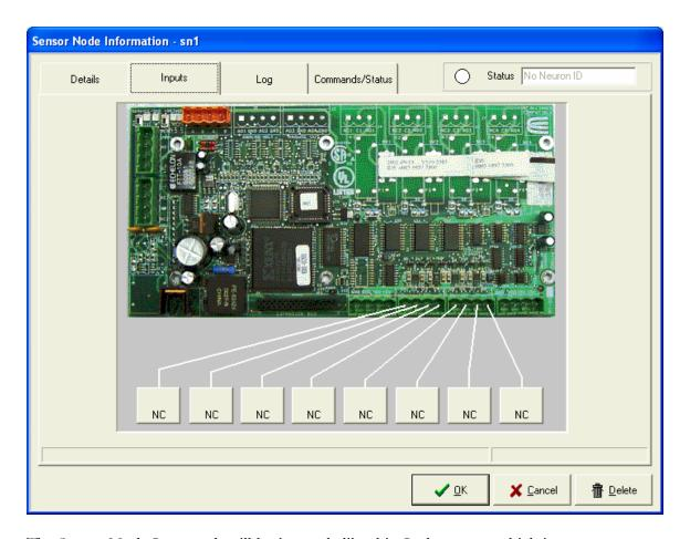
The Sensor Node Inputs tab will look exactly like this. It shows you which inputs are free and which inputs are used. You will be able to assign sensors to these inputs only after you drop the sensors. Assignment is bi-directional. You can come here and click on the inputs to assign a sensor or you go on the sensor to select the alarm sensor node and input.
