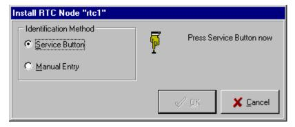
Press the Service Button on the RTC node or manually enter the Neuron ID. The proper software then gets loaded in the node, the node is commissioned, connections are made and configuration parameters are sent. The node is now fully operational. All nodes install exactly the same way. For more information on the other buttons and when to use them, refer to the 'Volume 2: Node Installation'.
