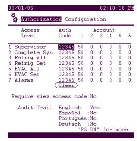
Note that there are 7 Access levels. Auth codes are assigned individually to each level,. Each level can have from 1 to 66 accounts.
