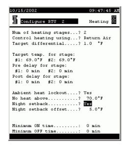
Num of heating stages Control heating using (0 to 3) The number of stages of heat in the unit. (List box:)
