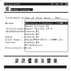
Any of the modem settings can be changed from this screen. Make changes with care, because incorrect modem settings can keep the system from communicating.
