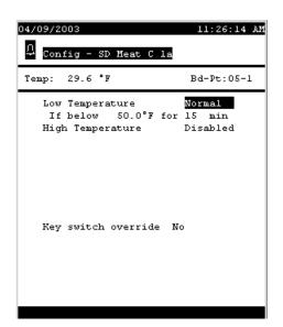
Notice that the name of the circuit appears in the heading of the screen. Then there is an area where the current sensor temperature appears, along with the number of the I/O board and point to which the case temperature sensor is wired. At first, you see two alarms, both disabled.
