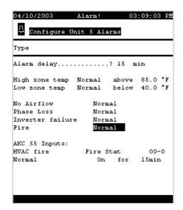
Notice the common alarm delay at the top of the screen. It can be set to any number from 0 to 100. The units, minutes, can not be changed. The alarm types are:
