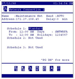
The address required is an IP address, and is the address of the ethernet node to which alarms are to be sent. The IP address is assigned by your network administrator. The address is composed of four one-, two-, or three-digit numerals separated by periods. None of the groups can be a number greater than 254 or less than 1.
