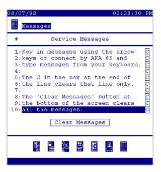
Instructions for use of the message screen are shown in the illustration above. Remember to toggle edit mode for each line by pressing the +/- key, and press ENTER at the end of each line.
