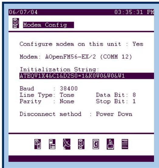
Fig. 15 The modem settings screen
