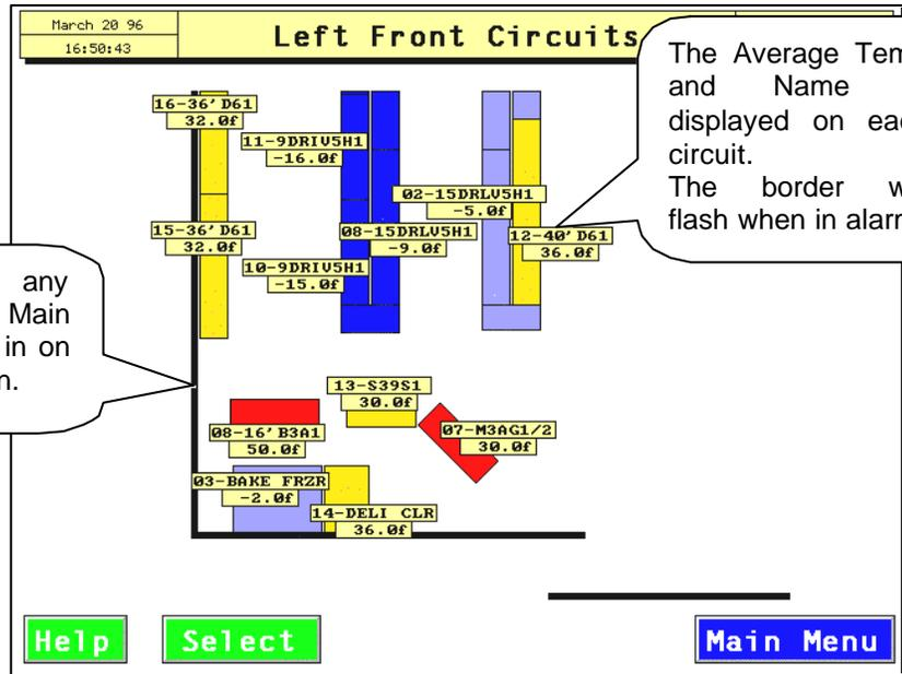
The Average Temp and Name is displayed on each circuit. The border will flash when in alarm.
