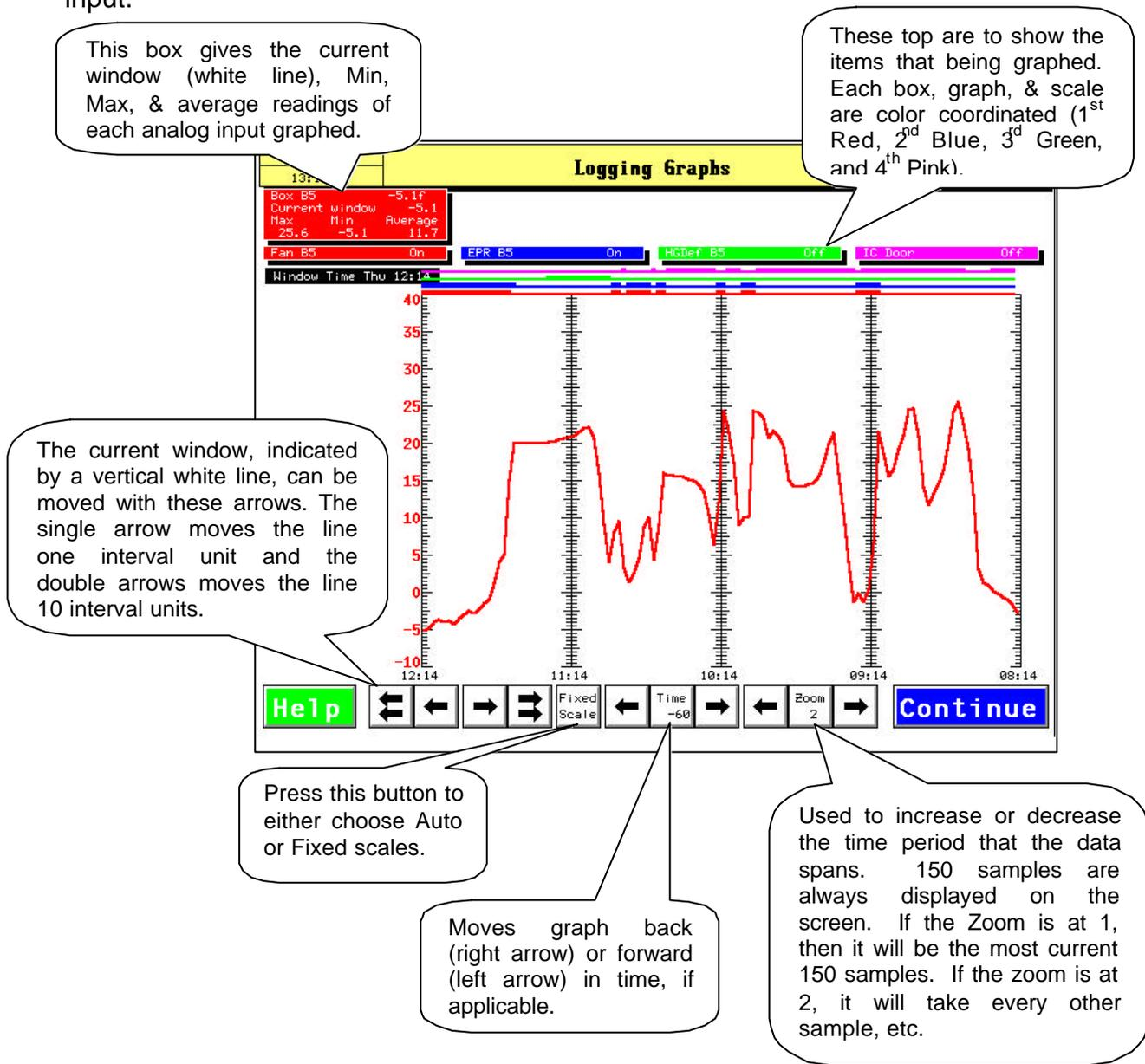
This box gives the current window (white line), Min, Max, & average readings of each analog input graphed.
