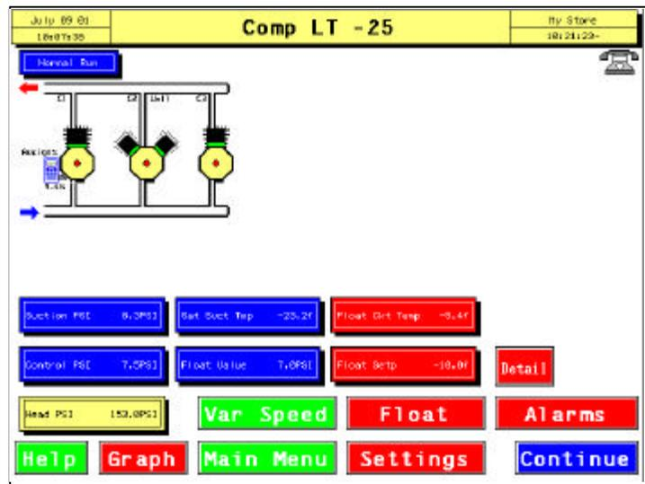
For variable speed, the accumulator value and the percent speed output is shown next to the inverter icon - the accumulator value being on the bottom and the speed on the top.
