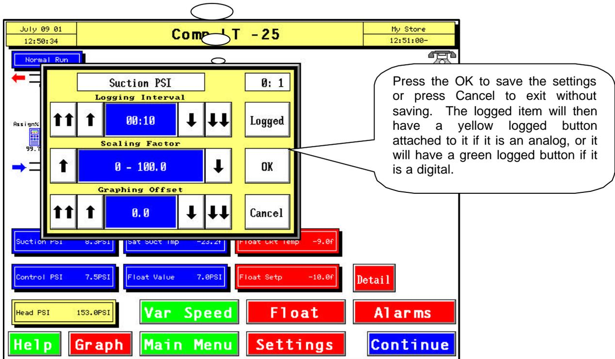
**Logging Interval** sets the time between samples; it defaults to 10 minutes but may be adjusted up or down by touching the arrows. The single arrow moves the value one minute at a time, the double arrows move the value in 30 minute increments.
