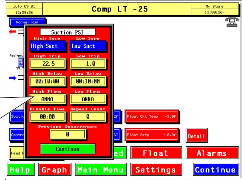
If the High or Low Flag buttons are pressed another panel will pop-up next to the alarm panel to allow the flags to be changed. An example of this screen follows:
