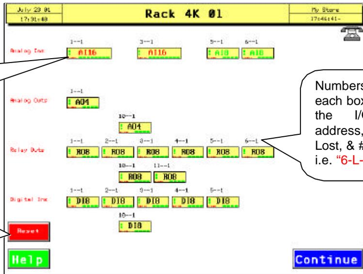
Numbers on top of each box represent the I/O board address, "L" for Lost, & # of errors. i.e. "6-L-250"
