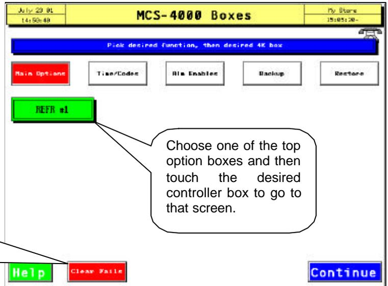
"Clear Fails" manually tells the ADV-6000 to rescan for known controllers that may have lost communications. Often used after a system PM or repair.
