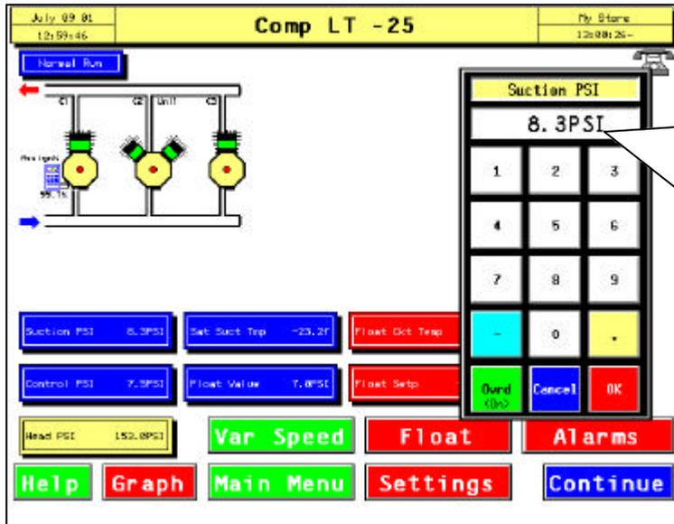
To set a manual /override value simply type in the desired value, then touch the "Ovr" button and toggle it to (On), press OK to save the change or Cancel to void the entry. To remove the override simply touch "Ovr" again to change it to (Com) and press OK.
