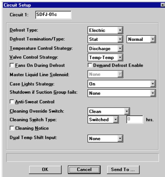
All case control circuits defined within the controlled system are set up at the Circuit Setup screen.
