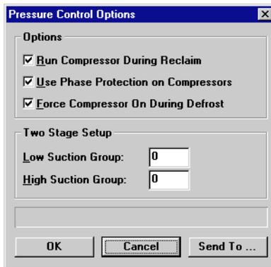
**Pressure control setup information is specified in the Pressure Control Options dialog box.**
