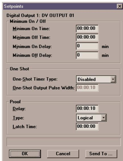
**All fields necessary to set up the Min On/Off, One Shot, and Proof cells are in the Setpoints dialog box.**
