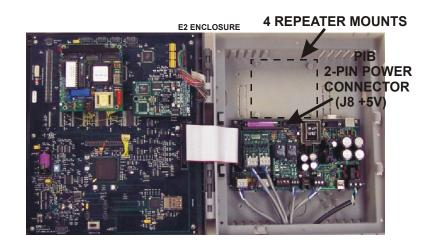
repeater. To terminate, move the jumper over the first two pins in the direction of the arrow. Refer to the table below for the termination jumper to use for
