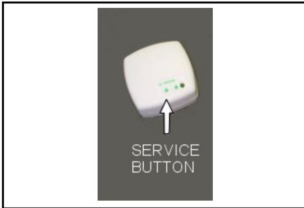
Figure 4-6 - VeriTemp Sensor Activation
