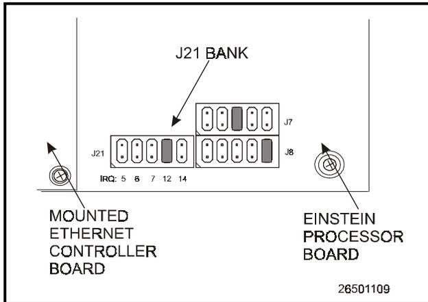
Figure 1-3 - Einstein Jumper Setup
