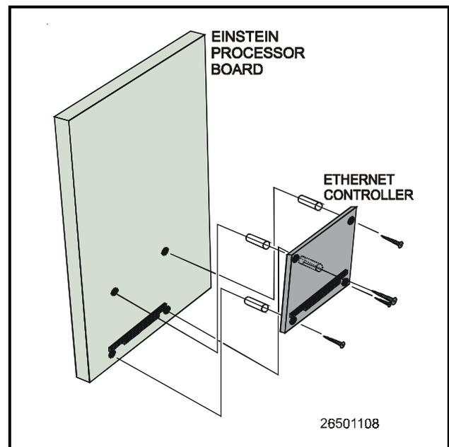
Figure 1-1 - Mounting Detail
