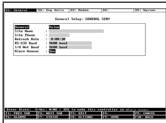
Figure 1-5 - Enabling Alarm Annunciator
