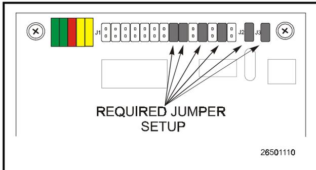
Figure 1-2 - NetCom Card Jumper Setup
