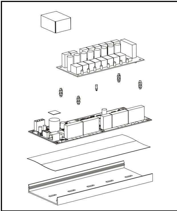
Figure 2-3 - Exploded View -- MultiFlex Combination I/O Board
