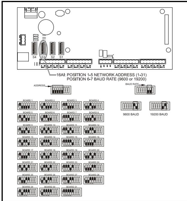
Figure 3-2 - 16 Network ID and Baud Rate Switches
