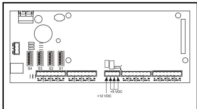
*Figure 4-2 - Input Board Power Sources*
