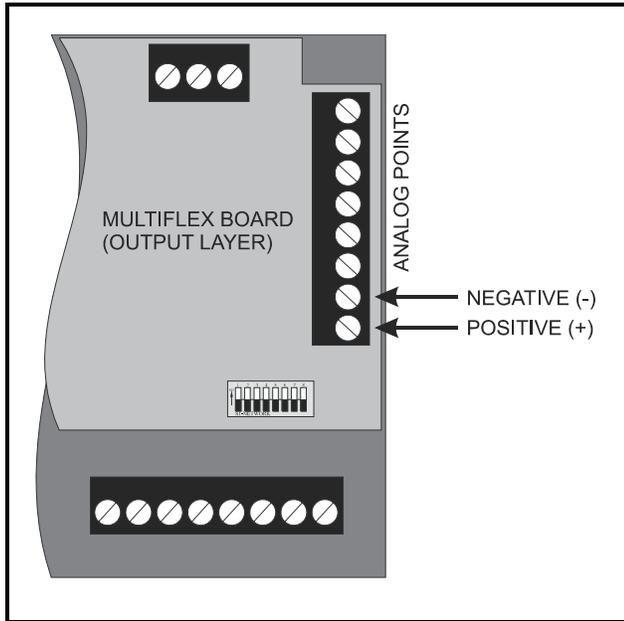
Figure 4-5 - MultiFlex Analog/Digital Points
