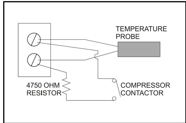
*Figure 4-3 - MultiFlex PAK Discharge Temp Point Proof Wiring*
