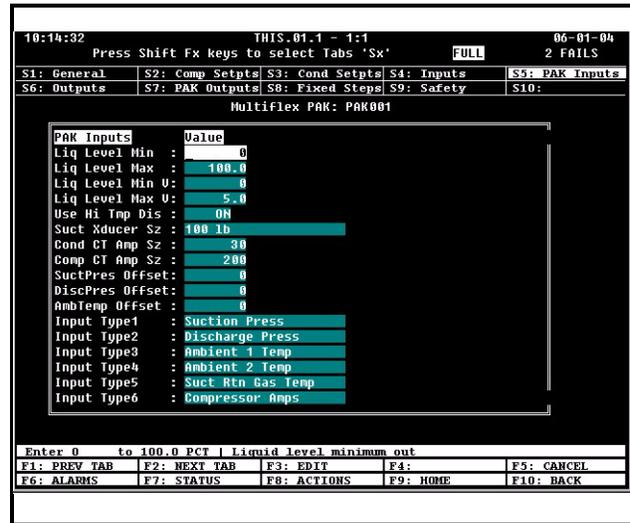
Figure 7-7 - PAK Screen 5: PAK Inputs
