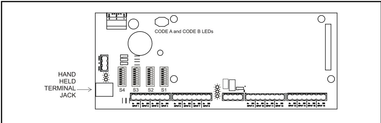
Figure 8-1 - MultiFlex HHT Jack Location
