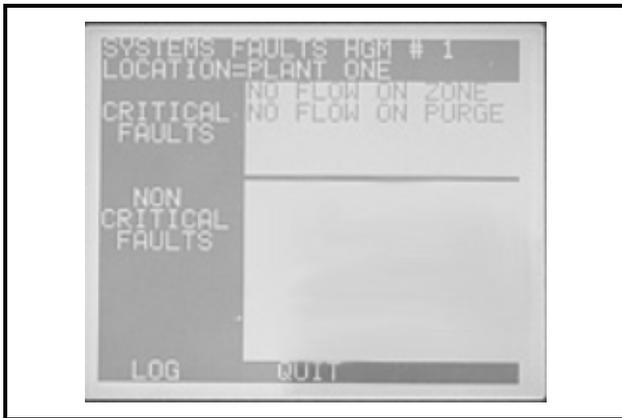
Figure 20-1 - Fault Screen
