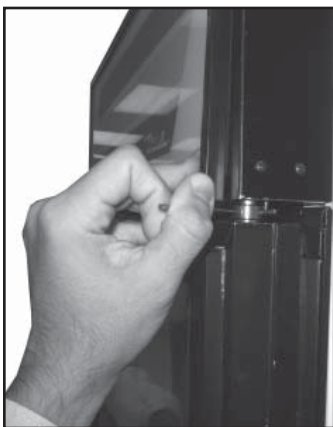
Image 1. (Releasing door tension).
