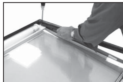
Image 4. (Removing door back plates).
