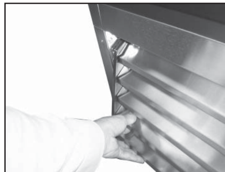
Image 1 (Removing two (2) lower screws then louvered grill hinges out then unhooks for removal).
