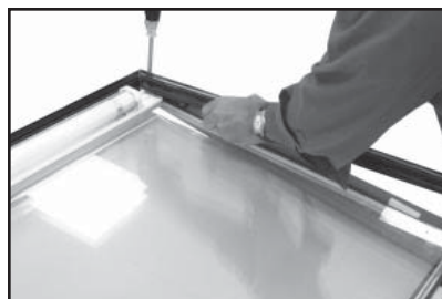
Image 4. (Removing door back plates).
