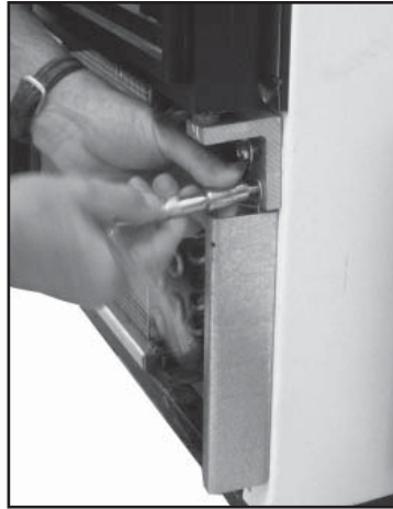
Image 2. (Removing door bottom hinge).
