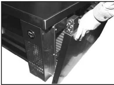
Removal of Side Grill
