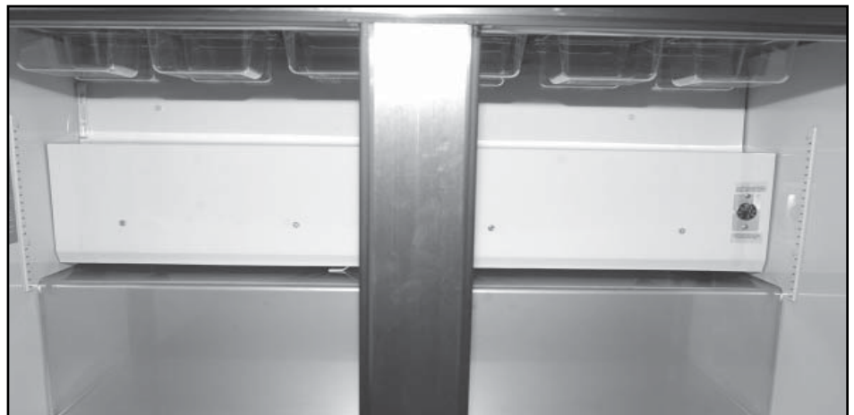
Figure 2. Removing evaporator lid.
