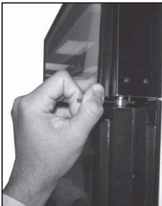
Image 1. (Releasing door tension).
