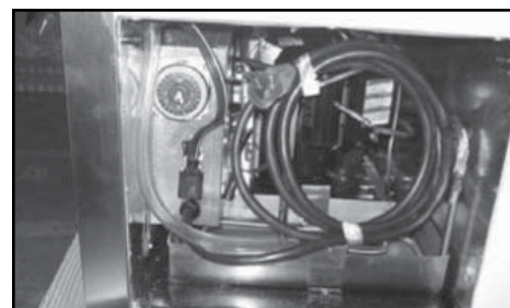
Image 3 (Defrost timer on TSID and TDBD-36/48 models).
