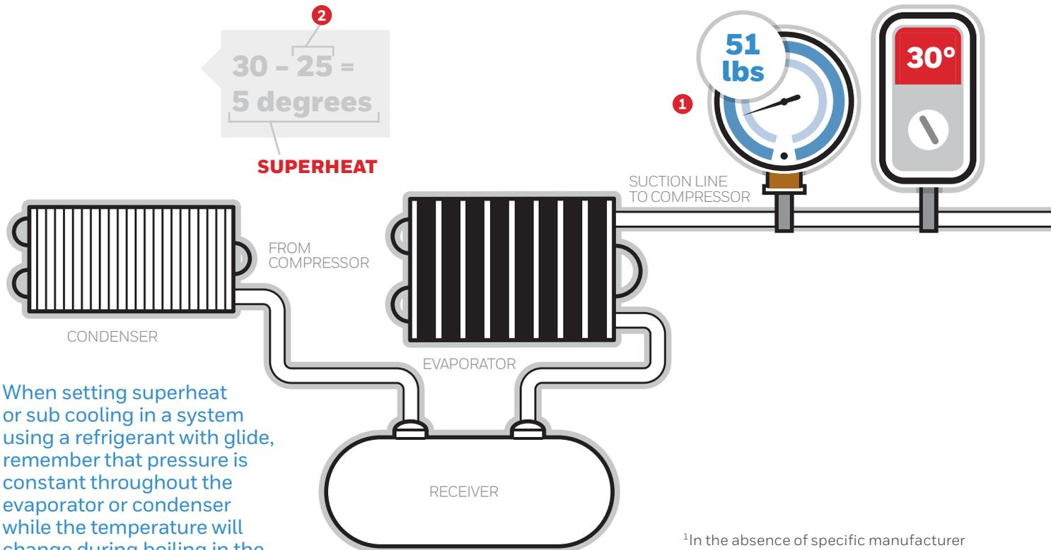
When setting superheat or sub cooling in a system using a refrigerant with glide, remember that pressure is constant throughout the evaporator or condenser while the temperature will change during boiling in the evaporator or condensing in the condenser.
