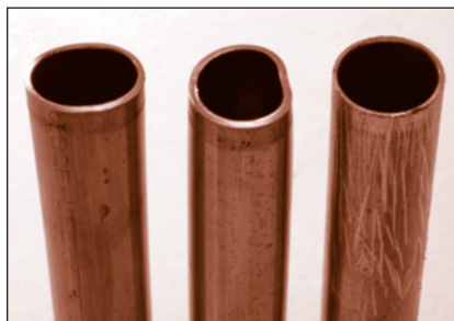
FIGURE 33: Inspect tube for imperfections
