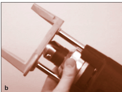
FIGURE 79 (a and b): Retracting the forming pins
