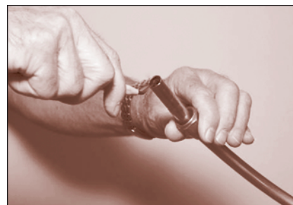
FIGURE 30: Reaming prior to flaring the tube end
