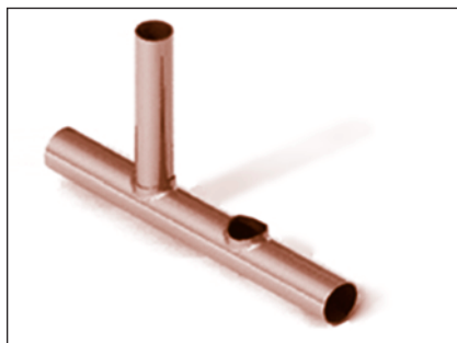
FIGURE 74: Mechanically formed extruded outlet requires only one brazed joint
