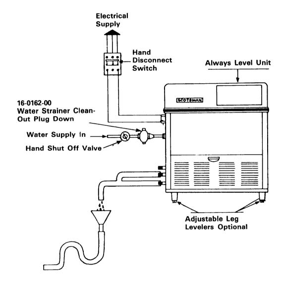
WATER SUPPLY. The recommended water supply line is 1/4 inch OD copper tubing. Connect to cold water supply line with regular plumbing fittings, with shut-off valve installed in an accessible place between supply line and machine. A water strainer must be installed with the unit and mounted with clean-out plug down. Locate the strainer next to the machine with the arrow in the direction of the flow. Most plumbing codes also call for double check valves in the supply water line.
