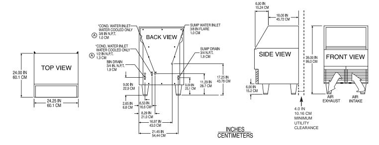
INSTALLATION NOTE: Allow 6" minimum space at back for utility connections.
