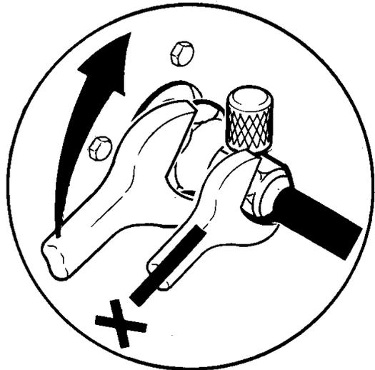
4. Using a marker or pen, mark a line lengthwise from the coupling union nut to the bulkhead. Then tighten the coupling and additional 1/4 turn. As the nut turns, the line will show when 1/4 turn is made.
