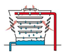
A cooling tower cools the condenser water by spraying it through a stream of ambient air. A schematic diagram of a cooling tower and the manner in which it servers the refrigeration condenser is shown. The air and water flow patterns suggested are counter-flow, a frequently used pattern. The key concept is that the leaving water temperature can approach the wet bulb temperature of the entering air.
